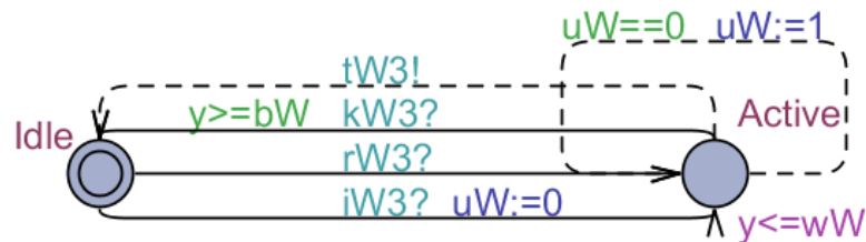
Figure C.10: Automaton core_3.W in the concrete model
