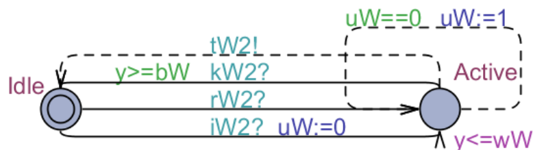
Figure C.8: Automaton core_1.W in the concrete model
